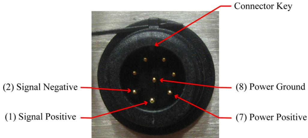
The connector is a Bulgin Buccaneer 400 series. The mating connector is part # PX0410/08S/6065 for 6.0 to 6.5mm diameter cables. Bulgin can supply other cable clamp fittings for other cable diameters. The connector is IP68 rated when mated or capped.
