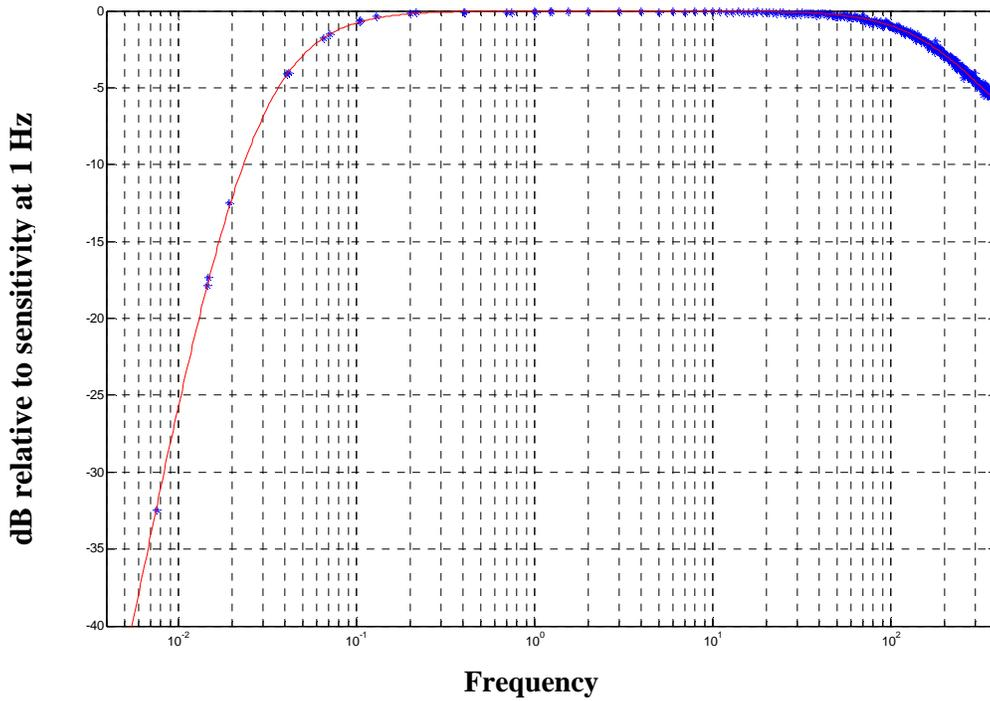
This plot shows the roll off at either end of the nominal 0.1-200 Hz band pass of the Model 20. The blue stars represent tests on Model 25 sensors. The red curve is the best fit of the data.
