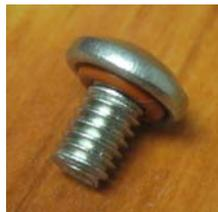
Vent Screw showing rubber o-ring
