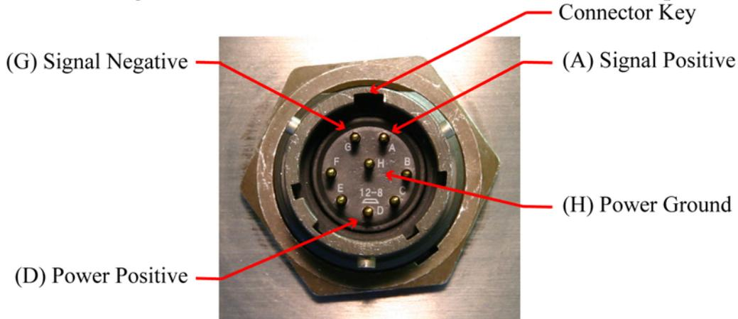
The connector is a PT07E-12-8P. The mating connector is a PT06E-12-8S-SR or a MS3116F12-8S; these two part numbers are functionally equivalent. This is an environmental connector and is sealed with or without the dust cap.
