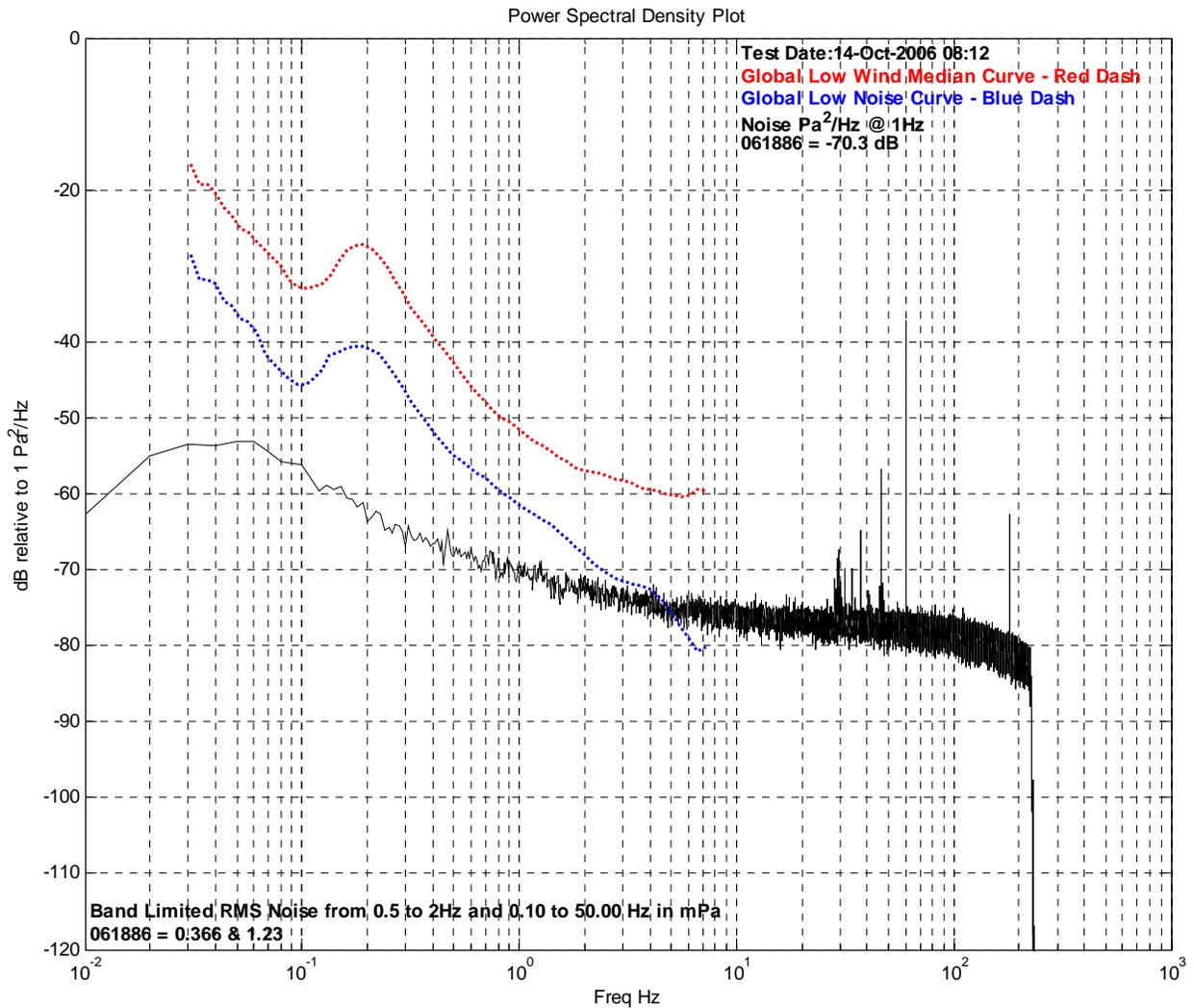
The black trace is from a Model 25 (sn061886) sensor in high gain with the acoustic inputs capped. The Mode 20 has the same noise curve. The spikes are from building vibrations and 60 Hz pickup. The self noise is approximately the same in both high and low gain once the output is converted to Pa. The red and blue traces are from data collected world wide. The red curve is a low wind median, while the blue curve is a 5% confidence lower bound for noise.
